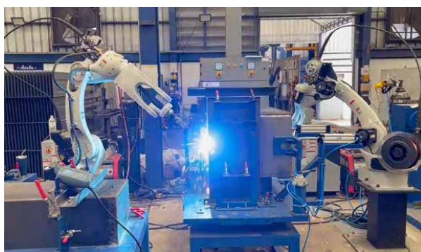
Sample Image of Welding to Assemble 300 kVA (MEA) Lids and 50 kVA (PEA) Tanks
