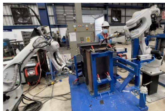
Sample Image of Welding to Assemble 300 kVA (MEA) Lids and 50 kVA (PEA) Tanks
