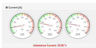
Example of Values Displayed in Smart Transformer Monitoring System V3.1 (Super Low Loss Transformer, QTC Factory)
